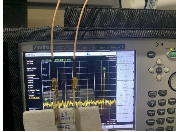
Fig. 5.12. Spectrum analyzer-based measurement setup for efficiency evaluation.
