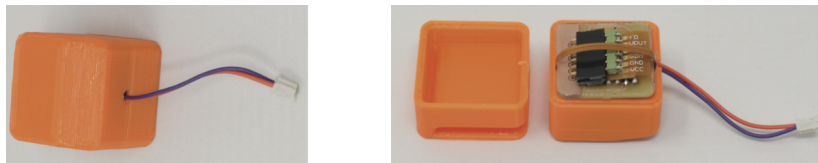
Figure 5.2: 3D Printed Casing Closed and Open View
