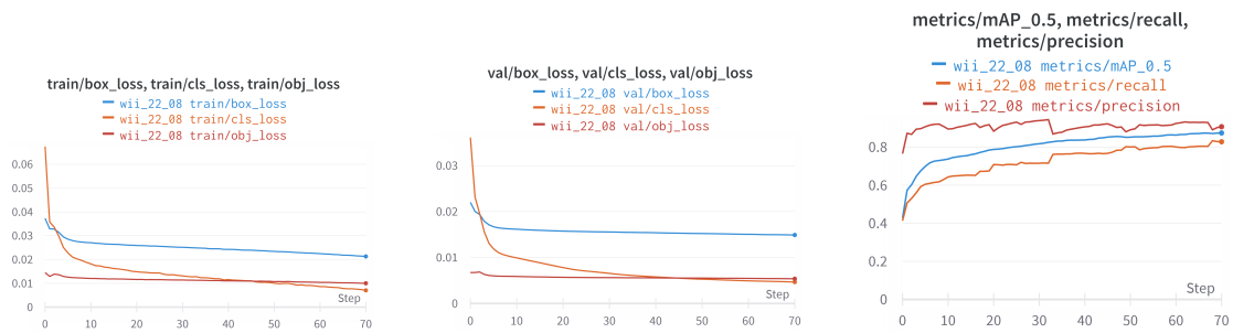
Figure 3.9: Train and validation loss plots along with mAP on the test set
