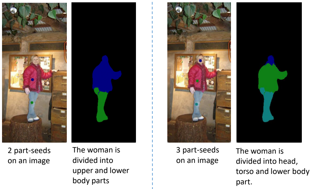
Figure 1.1: Interaction allows the user flexibility to decide how many parts he/she needs and at what level.
