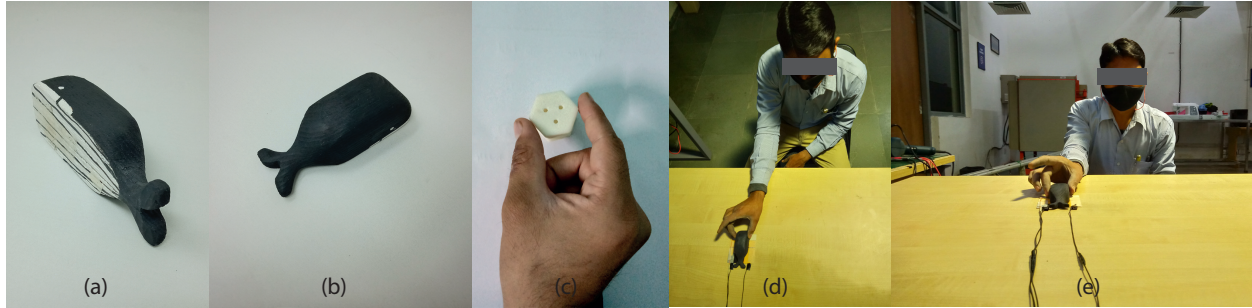
Figure 2.11: (a), (b) Fish object attached with HaptiDrag Pad used to slide pad over a surface; (c) Shows a two finger hand gesture adopted to hold fish object, and (d), (e): Shows real image of participant activity during a study
