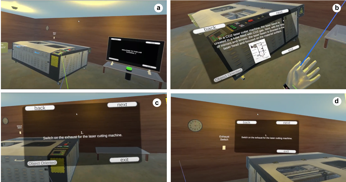
Figure 3.1: Four Spatial Representations for placement of learning content in VRLEs. (a) World-anchored: on a TV screen fixed in the environment. (b) User-anchored (Controllers): on a panel anchored to the VR controllers. (c) User-anchored (HMD): on a panel anchored to the head-mounted display. (d) Object-anchored: on a panel anchored to the object associated with current instruction.
