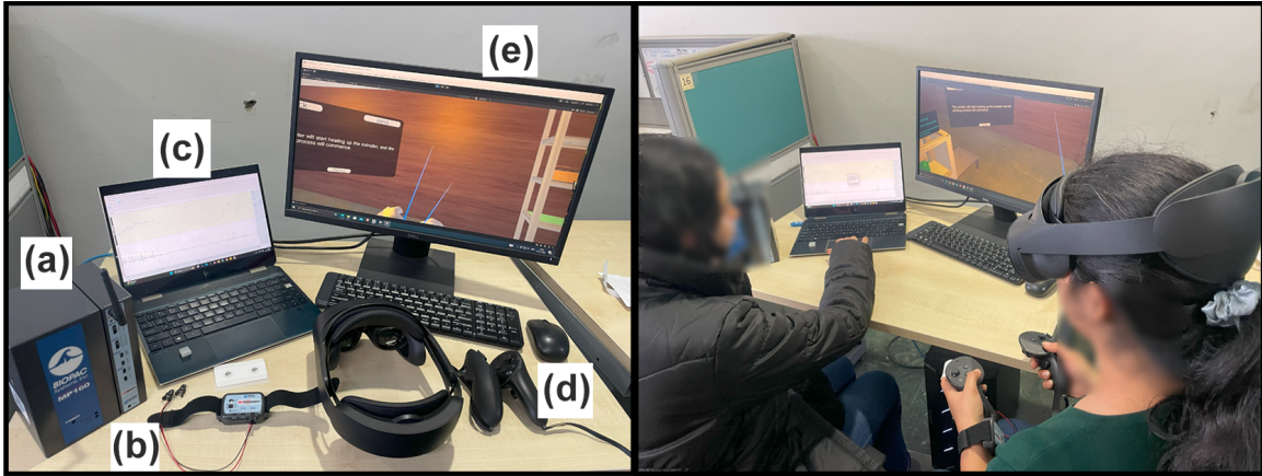
Figure 4.2: The left figure illustrates our experimental setup. (a) Biopac MP160 Acquisition System, (b) Wireless EDA sensors, (c) system with AcqKnowledge 5.0 running for EDA data collection, (d) Oculus Quest Pro VR headset and (e) system connected to headset via airlink for screen recording user interaction with tutorial. The right figure shows a participant performing the experiment.
