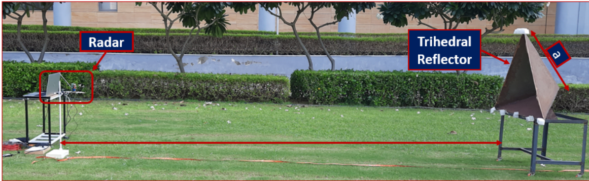
Figure 3.1: Experimental setup to calibrate the mm-wave radar at 77GHz using a trihedral corner reflector as a calibration target of known radar cross-section.
