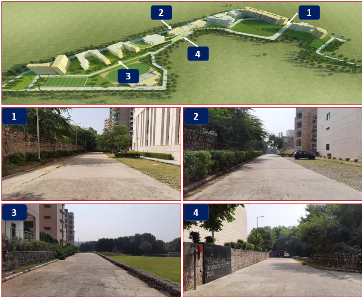
Figure 3.2: Different locations at which road surface clutter coefficient was estimated. Locations 1, 2, and 3 correspond to 7m wide concrete road, while location 4 is a 9m wide asphalt road.
