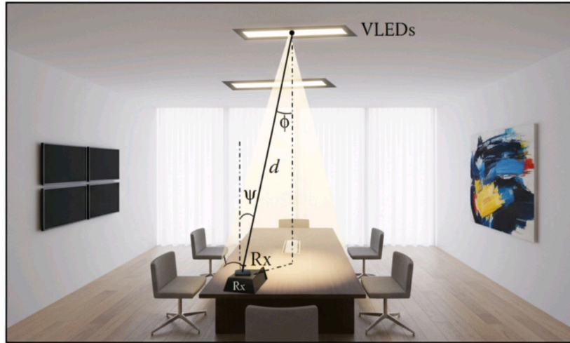
Figure 2.4: Li-Fi channel model.
