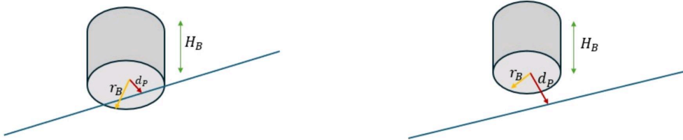
Figure 4.3: Geometric evaluation of blockage intersection along the LoS path.
