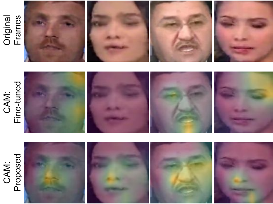
Figure 4.7: Class Activation Maps for some samples that are misclassified as real by the fine-tuned model but correctly classified by the proposed model. (a) is original image classified as Deepfake while (b) and © are Deepfake images classified as original.
