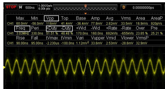
Figure 3.10: Time-domain response of the modified receiver.
