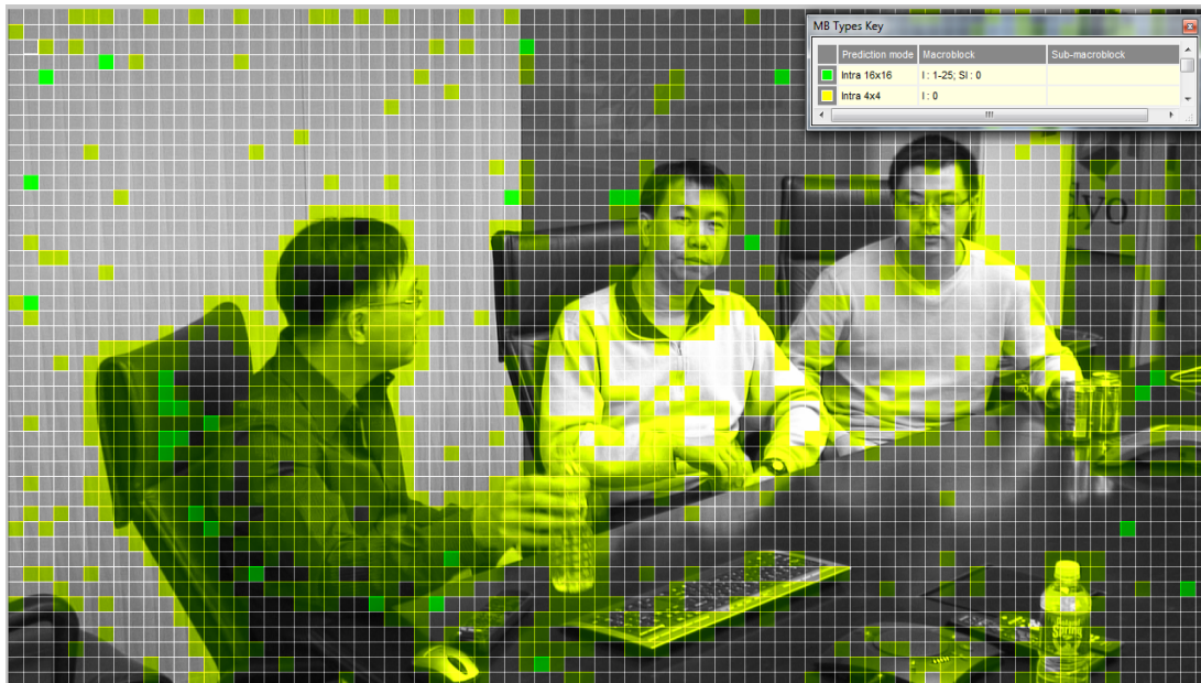
Figure 6.1: The snapshot of a frame of video sequence vidyo1_1280×720_60 encoded using the proposed algorithm
