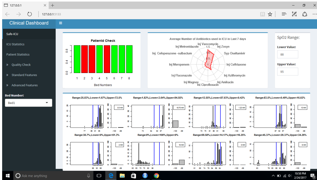
Figure 4.2: The dashboard front page, patient id check barplot, Radar plot of antibiotic used in last 7 days, oxygen saturation of each bed in last 1 hour with default range of 88 to 95
