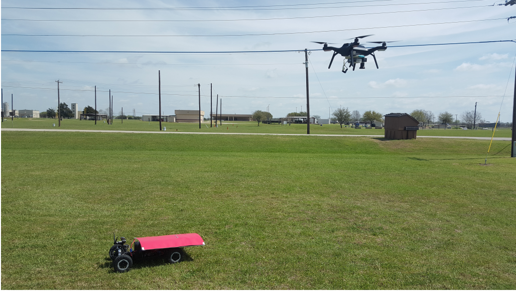
Figure 4.1: Hardware setup consisting of the quadrotor attempting to land on the target mounted on a ground rover. The quadrotor is equipped with a camera (point Grey Chameleon 3) and Odroid U3+ embedded computer
