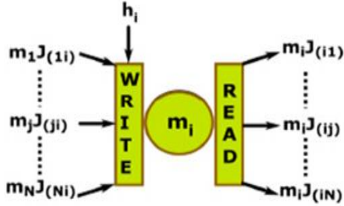
FIGURE 2.1: The interaction among individual p-bits is represented using distinct read and write units. Each p-bit m_i is influenced by a local bias ( h_i ) and some weight ( J_{ij} ) which couples the effect of all the neighbouring p-bits m_j 's on p-bit m_i . [1]
