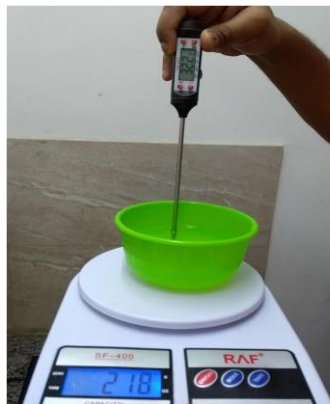
Figure 3.18 Weighing machine for the measurement of weight of phantom to be used in the determination of specific heat capacity (weight of empty container = 18g, total weight = 200 g (phantom) + 16 = 218g)
