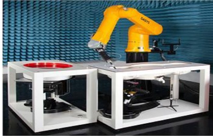
Figure 3.2 Practical electric field probe scanning method for the determination of SAR (DASY 6 by SPEAG) [72]
