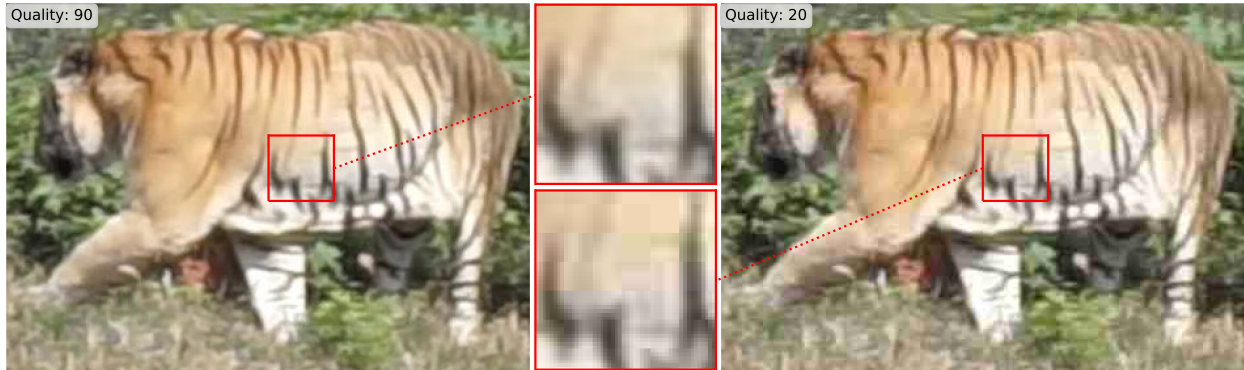
Figure 4.3 Effect of JPEG compression: At the lower quality (higher compression), block-like color artifacts introduced by the compression are visible. While this change may seem insignificant to the human eye, it changes the internal statistics of the image. Compressing the images at different random quality values during training helps the network become robust to those statistical differences. Given the fine-grained nature of this visual recognition problem, we saw significant improvements in our empirical analysis
