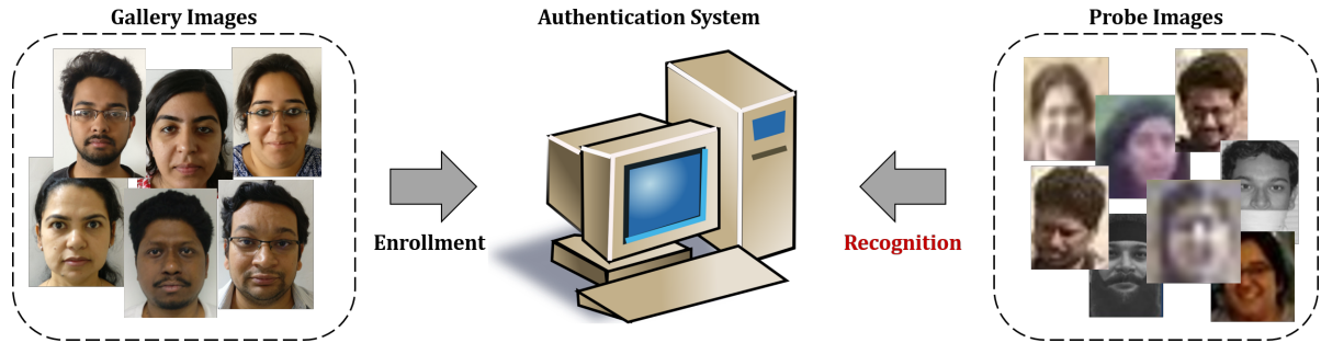
Figure 1-3: Often in real-world scenarios, the authentication system is developed using facial images captured in constrained environments. However, at real-time the system might encounter images captured in unconstrained scenarios with several covariates such as resolution variations or presence of disguise accessories. The authentication system must therefore be able to match the given input with the constrained gallery samples provided during enrollment.
