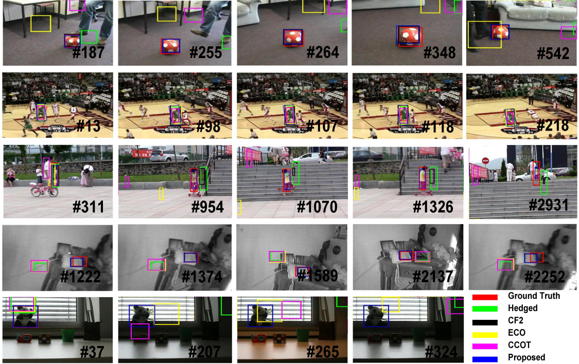
Figure 4.18: Intermediate Frames Showing Tracker’s Performance During Various Challenges: Row 1 - Size Change, Row 2 - Object Inclination, Row 3 - Occlusion, Row 4 - Shaking Camera, Row 5 - Illumination Variation. Proposed tracker is able to the track target during challenges where other trackers fail.
