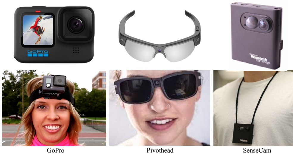
Figure 1.2: The figure demonstrates a few wearable devices with their installation on the wearer. GoPro, Pivothead, and SenseCam are head/hat-mounted, glass-mounted, and chest-mounted devices, respectively.
