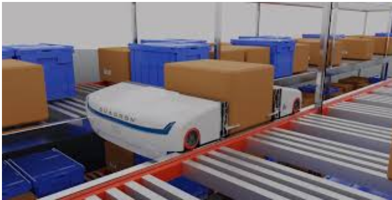
Fig. 1.4. Warehouse with smart ASRS System
