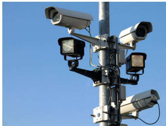
FIGURE 1.4: A typical multiple setup with several NIR illuminators to cover a large field of view. Image source: bbc.com, Image creator: Getty Images.
