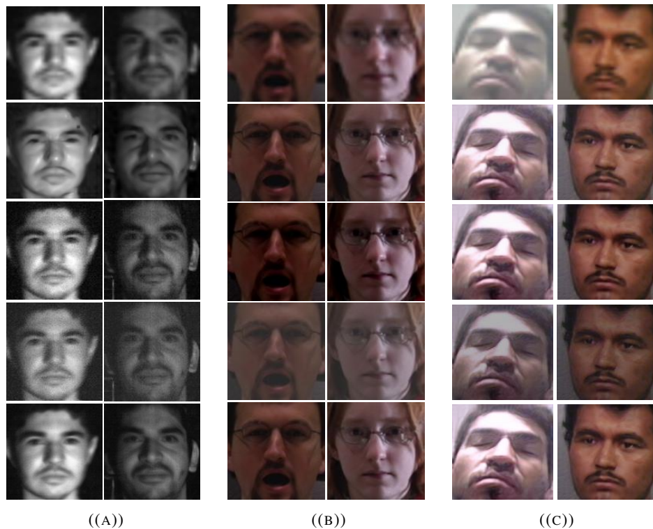
FIGURE 3.6: Translation of probe images from low to high resolution, showing enhancement in image quality, where (a) Images of FaceSurv database, (b) Images of CMU MultiPIE database and (c) Images of NIST MEDS database and first row: bicubic interpolated low resolution images, second row: images generated by Isola et al. [65], third row: images generated by Zhao et al. [140], fourth row: images generated by Choi et al. [141], fifth row: images generated by our proposed method. These translated images are then used for face recognition experiments.
