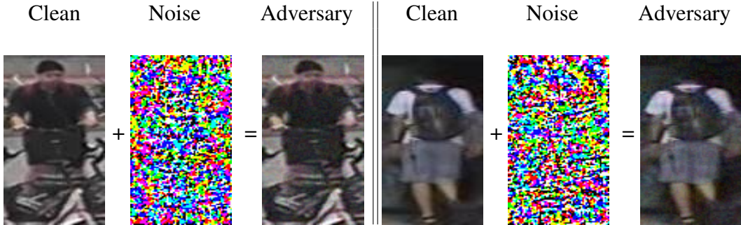
Figure 4.4: The figure illustrates the adversarial sample obtained by adding noise to clean images.
