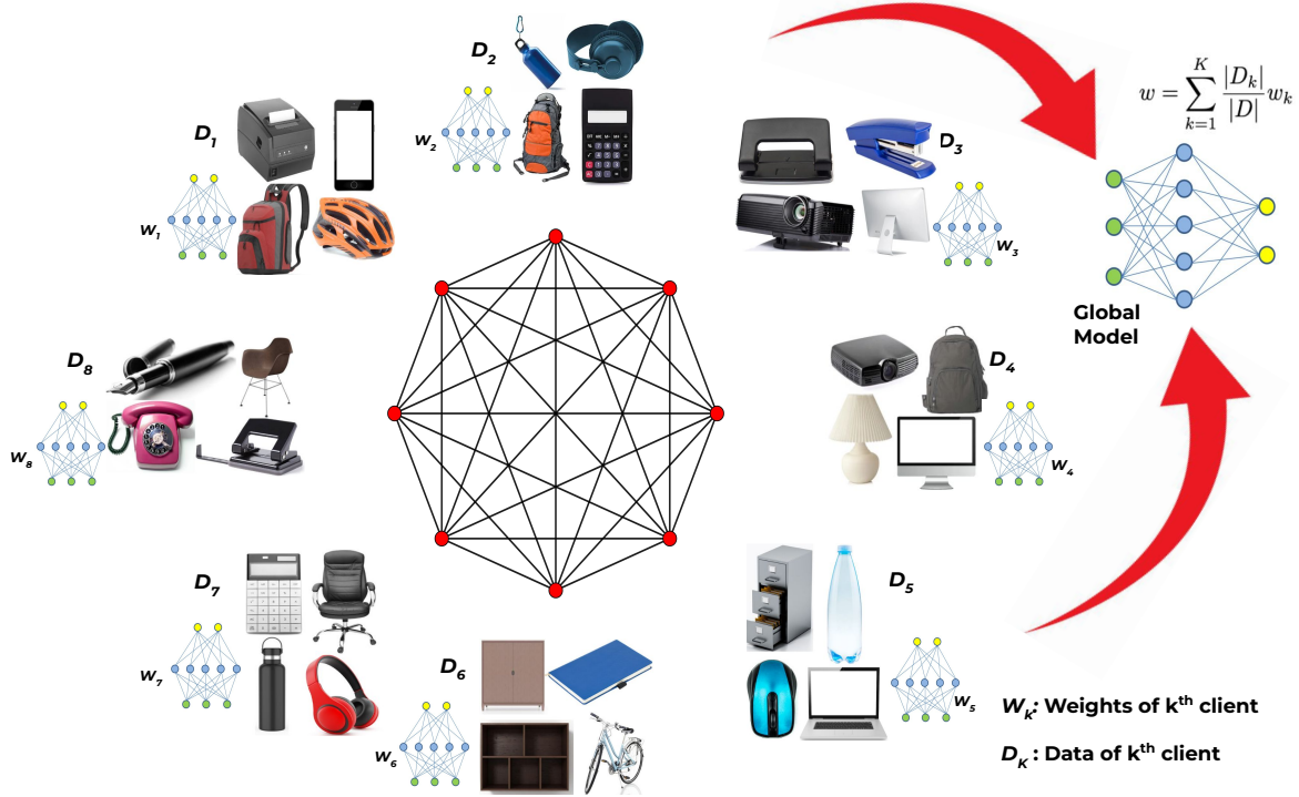
Figure 3.3: Proposed model using Fed-Star demonstrating pre-aggregation of the parameters in star topology manner among local clients and is given by equation (3.9). This is followed by the transferring of weight to the global model where aggregation of weights is performed.
