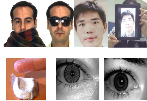
Fig. 1. An illustration of some known vulnerabilities for face (masks), fingerprint (gummy prints 1 ) and iris (color/textured contact lens) biometrics at capture phase.
