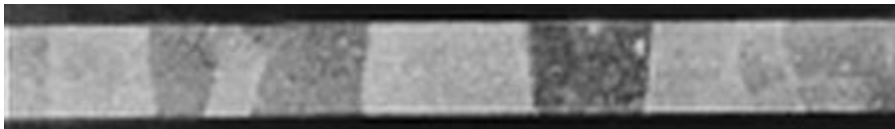
Figure 10: A Metal Lines in Which Grains Are Perpendicular To The Track. As The Flowing Electron Does Not Find The Disordered Grain Boundaries, There Is No Electromigration.
