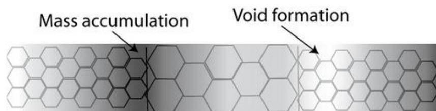
Figure 9: When The Atoms Moves From Fine-Grained Region To Coarse Grain Region, Hillocks Are Formed And When The Atoms Moves From Coarse Grain Region To To Fine-Grained Region, Voids Are Formed.
