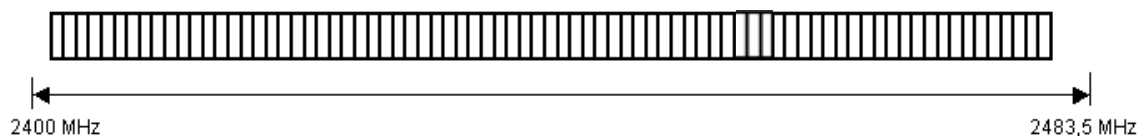
Figure.8 Bluetooth operating band with 79 channels for frequency hopping
