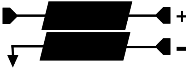
Fig. 1.3. A capacitively coupled transmission line type balun
