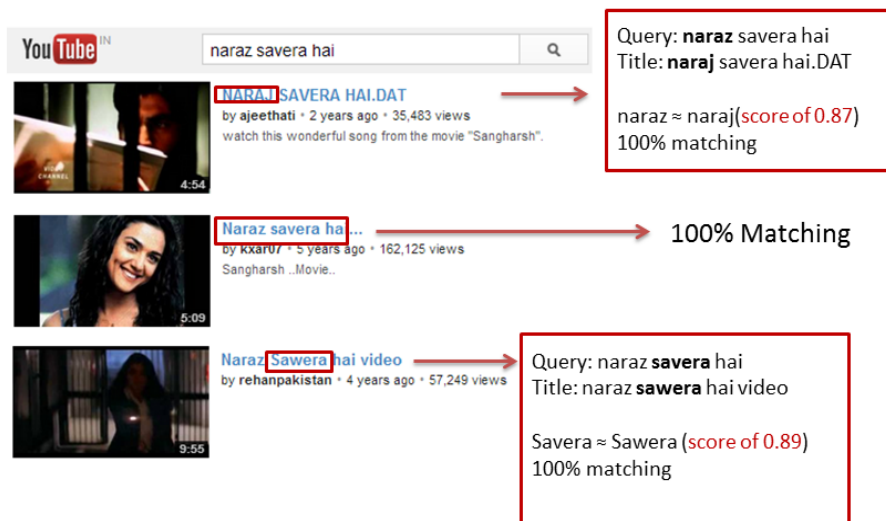
Figure 4.6: This snapshot illustrates an example of Textual similarity of video title to query.
