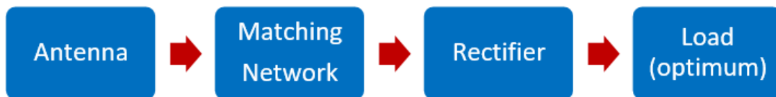
Figure 2.3 Block diagram for RF energy scavenging system.
