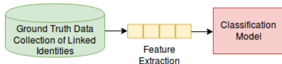
Figure 4.1: Basic Framework for User Identity Linkage which comprises collection of ground truth linked identities, feature extraction, and construction of classification model.
