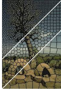
Figure 1.1: Figure shows 3 different sizes of regions from small to large differentiated by two lines as shown in [2]. In each region the intensity of pixels do not vary by a significant amount.
