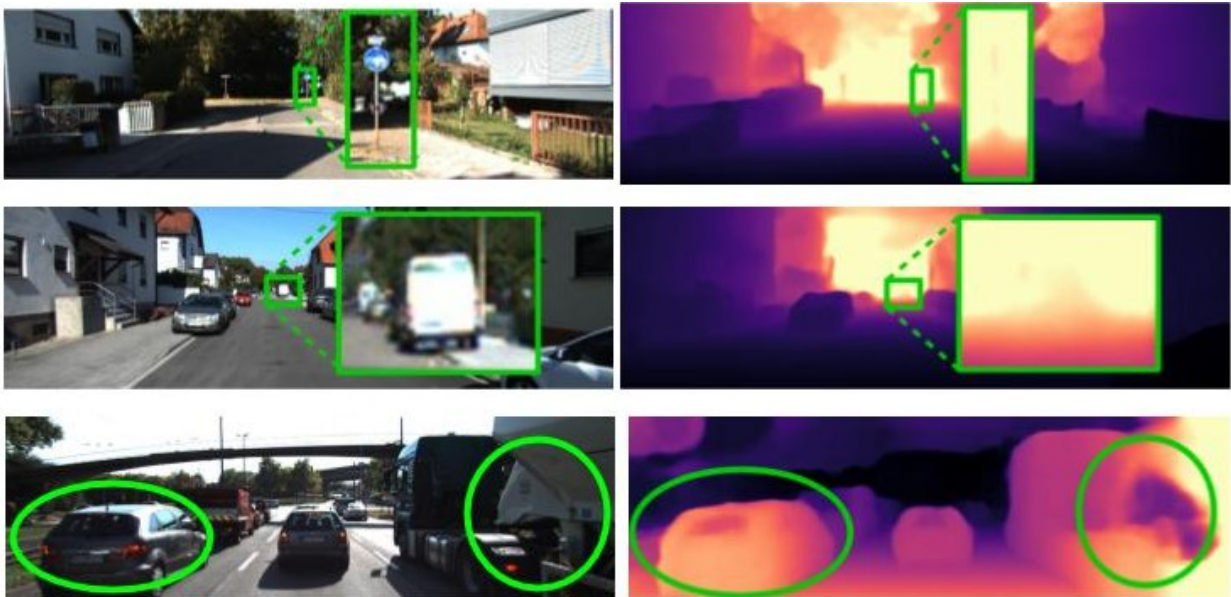
Figure 2.2: State-of-the-art unsupervised monocular depth prediction method MonoDepth2 [56] fails to predict accurate depth values for both the farther away points (top 2 rows) and also nearby points (bottom row).
