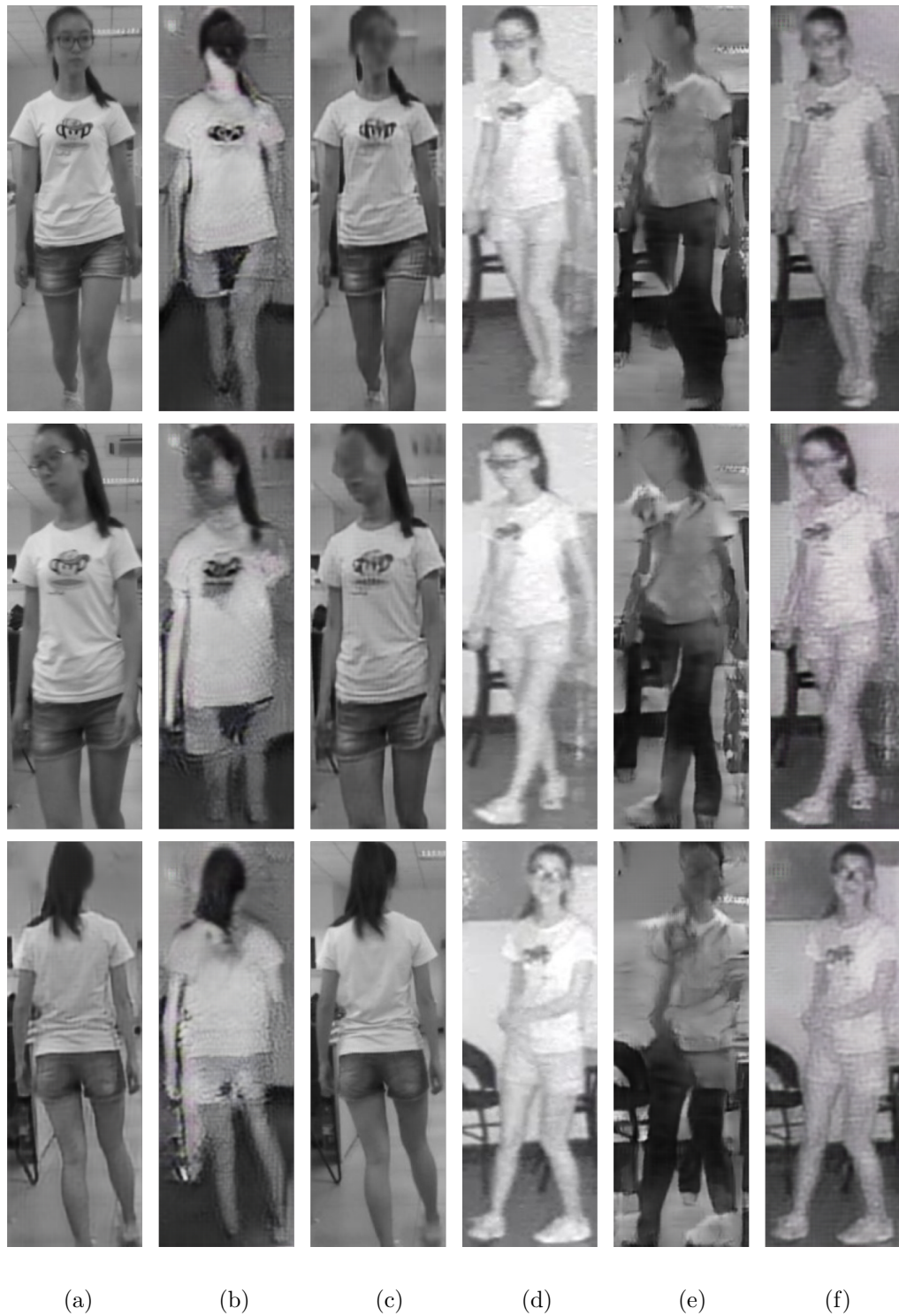
FIGURE 4.3: Final results. (a) Real grayscale Image, (b) Fake IR image, (c) Recovered grayscale image, (d) Real IR image, (e) Fake grayscale image (f) Recovered IR image
