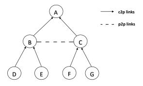
Figure 1: Schematic AS graph with multiple valid valley-free paths: D - B - E, D - B - C - F, D - B - C - G, D - B - A - C - F, D - B - A - C - G, E - B - A - C - F and E - B - A - C - G. Note how some do not traverse A, the AS with the highest customer-cone size.
