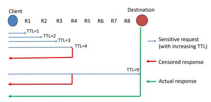
Figure 4.1: Iterative Network Tracer: Client sends a crafted query (DNS query/HTTP GET request) containing a blocked domain with increasing TTL. Censorship response is observed from the censor's network element.
