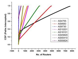
Figure 3.4: CDF of traceroute paths intercepted by individual routers, sorted by increasing number of paths through each router (for 8 important ASes.)
