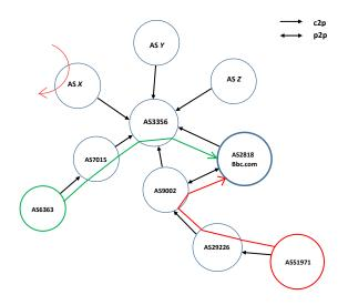
Figure 2.7: Valley free paths in the cone of AS3356. Green line: network path that traverses AS3356 to reach AS2818 directly. Red lines: network paths that traverse the one-hop customers of AS3356, but not AS3356 itself.
