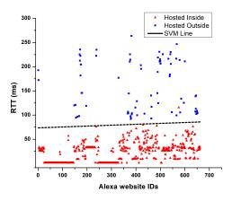
Figure 8: RTT scatter plot for a probe in Brazil.
