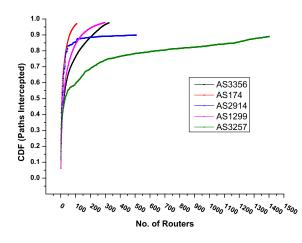
Figure 5: Traceroute paths in the top five (out of 30) key ASes. The number of routers needed to cover 90% of the paths varies between 288 (AS174) and 1483 (AS3257)
