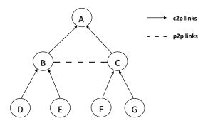
Figure 2.6: Schematic AS graph. A is "root" of customer cone.
