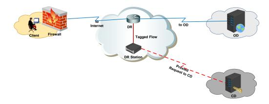
Figure 5.1: Decoy Routing in Action: Clients in a censorious ISP bypass the filter by sending packets apparently addressed to a non-filtered overt destination (OD). En route, the packets traverse a DR, which sees the secret message; identifies them for special handling; decrypts them; and sends their payload to the real, covert destination (CD).
