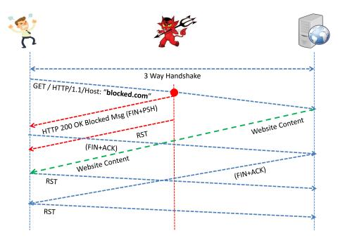
Figure 4.4: Censorship mechanism of a Wiretapping Middlebox.
