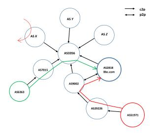
Figure 5.10: Valley free paths in the cone of AS3356. Green line: network path traversing AS3356 to reach AS2818 directly. Red lines: network path through one-hop customers of AS3356, but not AS3356 itself.
