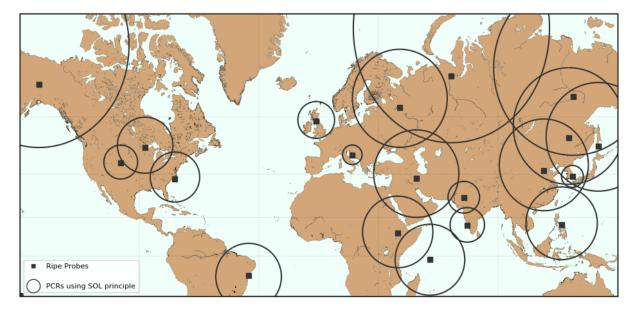
Figure 6.4: Detecting IP anycasting. Dots represent the RIPE probes and circles represent the distance estimated to the IP address based on speed of light constraint.
