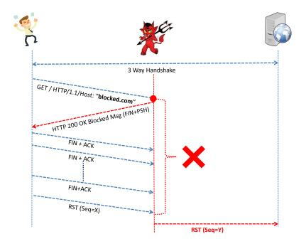
Figure 4.3: Censorship mechanism of a Interceptive Middlebox.
