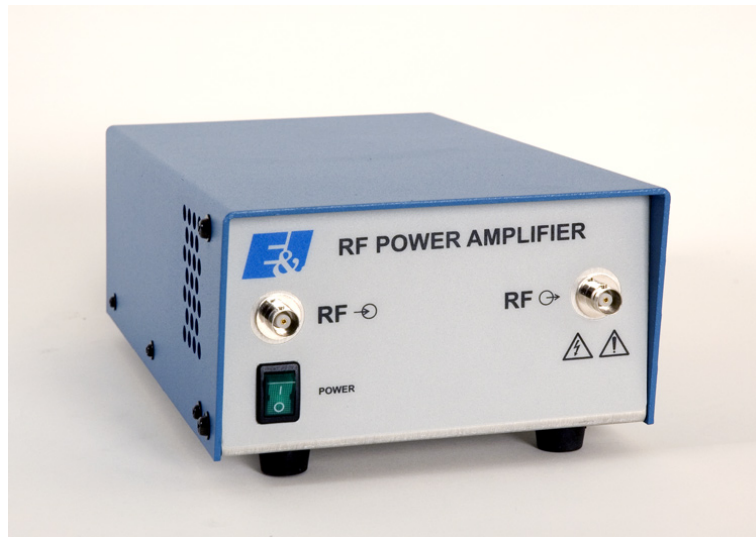
Fig. 1.23 3W power amplifier from acquitek
