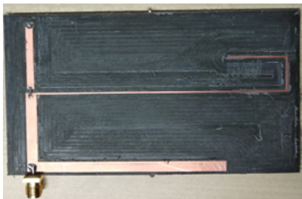
Fig. 3.17 Fabricated prototype with load-A @ 1 GHz: Load A- 50+j80
