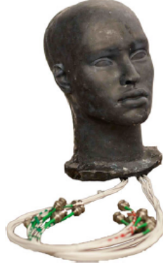
Figure 2.4: Complete Skull Phantom[27]
