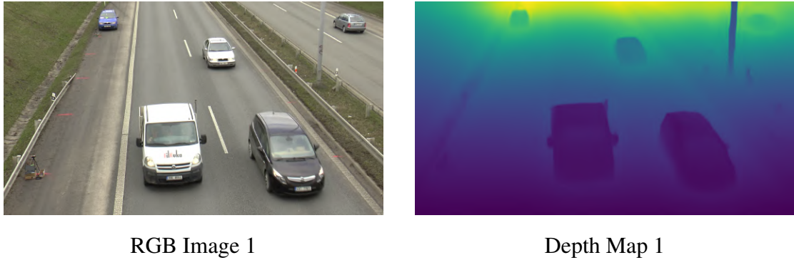
Figure 4.4: RGB images and corresponding monocular depth predictions using our depth estimation module.
