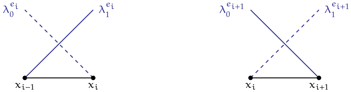
FIGURE 2.4: Elemental view of linear Lagrange basis in 1d.
