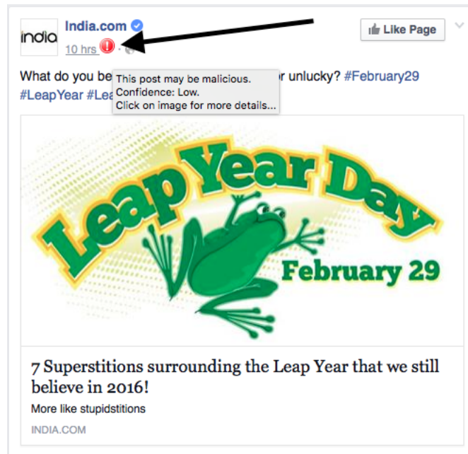
Figure 4.2: Sample Facebook post marked as malicious by Facebook Inspector. The small red image next to the time of post indicates that the post may be malicious. Hovering over the red image gives additional details to the user.
