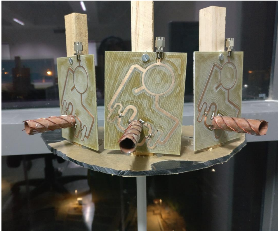
Figure 3.15: Receiver setup with three antenna elements.
