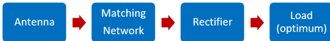
Figure 1.6 Block diagram for RF energy scavenging system.
