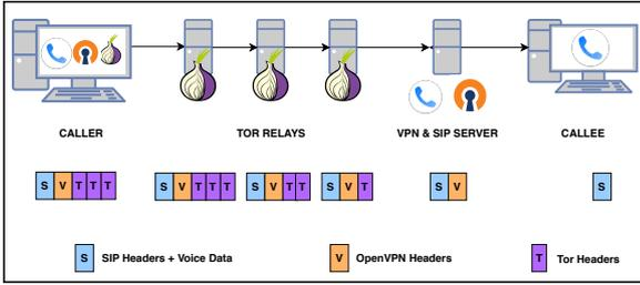
**Fig. 2. V-Tor:** The caller establishes a VPN tunnel through Tor, so that all the UDP VoIP traffic traverses the Tor network. On reaching the VPN server, the traffic is sent to the SIP server, which initiates a voice call to the callee.
