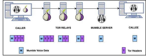
**Fig. 3. M-Tor:** The caller configures the mumble client to work in TCP mode. Thereafter, mumble’s traffic is sent over Tor eventually reaching the mumble server, which handles the call procedure between the caller and callee.
