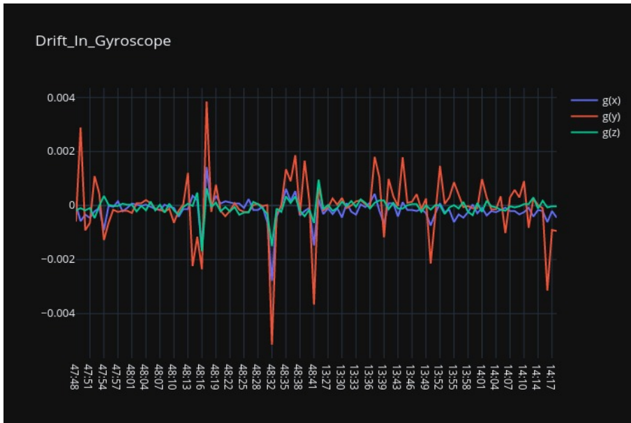
Figure 3: Drift Present In Gyroscope In Position 2
