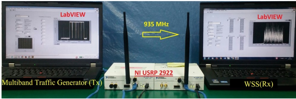
Figure 3.8: USRP testbed for validating the proposed learning and decision making algorithms.
